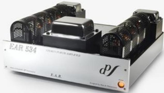
A Push-pull power amplifier with 50 watts per channel stereo utilising eight EL34 (four per channel) into 4, 8 and 16 ohms.
